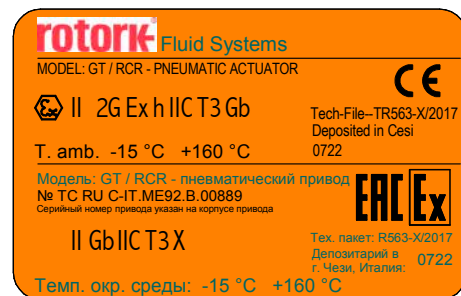
Fig 5.3 Actuator ATEX/EAC label for high temperature (-15°C<T<+160°C)
