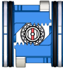
Fig 10.2 Assembly A – Clockwise to close actuators, upper shaft perpendicular to body
