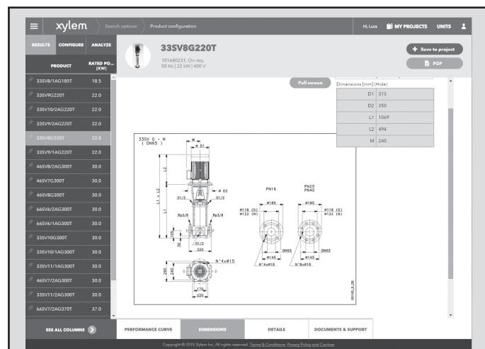
Dimensional drawings appear on the screen and can be downloaded in dxf format.
