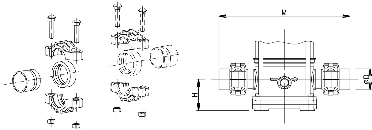
The single Kit includes: One cast iron Victaulic coupling with one AISI 316L stainless steel weld-on or threaded sleeve with EPDM or FPM gasket.
