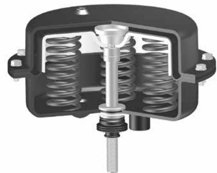
DP-Actuator Retracted stem on air failure
